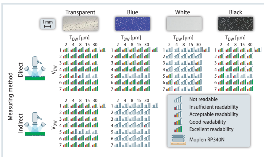
Fig. 4. Results of the readability of the digital watermark as a function of the application parameters and the molding compound color Source: Barnes Molding Solutions; graphic: © Hanser
